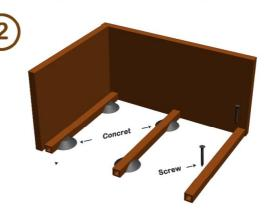
Two ways to fix the Joist: 1.Concret 2. Screw
