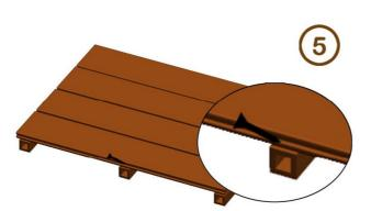
fix the decking and joist with screw from the side groove and in the middle length of decking, Each decking will only need to fix one point.
