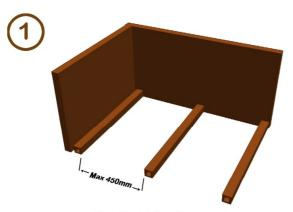
Place the joist on the ground Joist Span: 450MM
